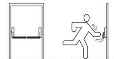
Figure 2 — Panic exit device with type A bar operation (push-bar)
