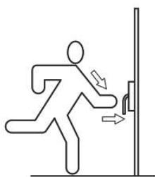
Figure 2 — Panic exit device with type A bar operation (push-bar)
