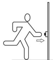
Figure 3 — Panic exit device with type B bar operation (touch-bar)
